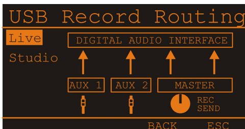
Turn the MENU/ENTER rotary encoder to select the assignment of CMS busses to channels USB 1 to 4 of the DIGITAL AUDIO INTERFACE. Following table lists the available assignments. Press the MENU/ENTER rotary encoder to apply the selected assignment. Pressing the BACK function key returns to the menu. Pressing the ESC function key discards all changes and returns to effect mode.
