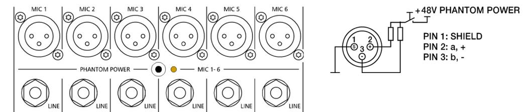
The MIC input accepts levels between -60 dBu and +21 dBu – depending on the setting of the corresponding gain control. Because of the low impedance and the switchable PHANTOM POWER the XLR input is preferred for MIC applications. Because of the high input acceptance of up to 21 dBu the XLR input is also suited to connect further mixers, effect units, keyboards etc. But because of the higher level and impedance matching the LINE input should be preferred.
