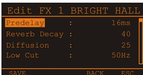
Turn the MENU/ENTER rotary encoder to highlight an entry in the left column of the Edit FX Menu. Press the MENU/ENTER rotary encoder to select the corresponding value in the right column. Now turn the MENU/ENTER rotary encoder to edit the value. Press the MENU/ENTER rotary encoder again to return to the left column. Press the SAVE function key to store the edited effect as a user preset. The FX User Presets dialog appears.
