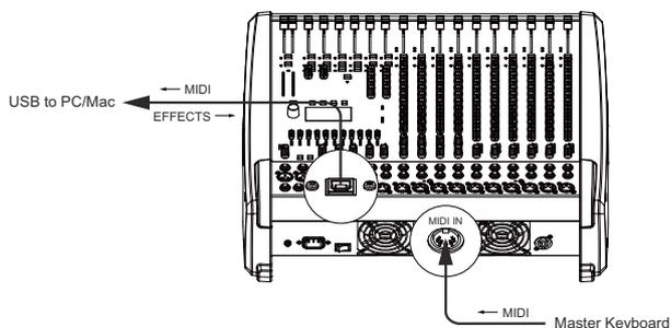
The CMS offers similar options for the creation of sound effects. The PC serves as an external, extremely powerful multi-effects unit. Since the signal is fed from one or both AUX ways, the operation during mixing becomes as simple as using the internal effects of the CMS. The AUX ways should be switched to post-mode. The effect signal generated in the PC is again added to the overall mix via USB stereo channels 1-2 and 3-4. The stereo channel faders serve as FX-return controls.
