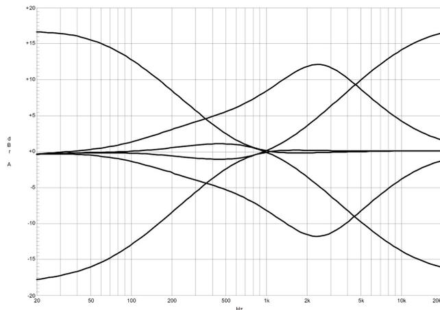
The EQ section of the STEREO channels is designed in a way that HI and LO controls provide a degree of control that is equally adequate for LINE level inputs and microphones. The MID control is active in a comparably wide frequency band around 2.4 kHz. With most microphones this is the critical range, where a slight attenuation offers excellent results.
