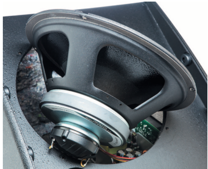
Coax system with neodymium compression driver for the high frequencies mounted
