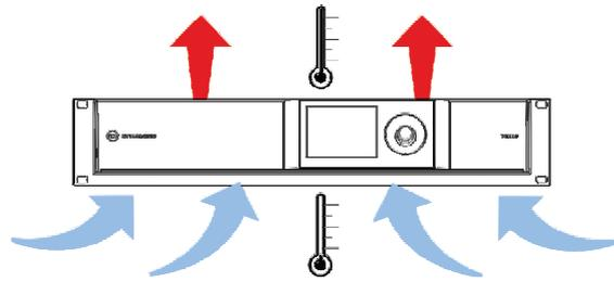
Figure 5.1: Power amplifier ventilation
