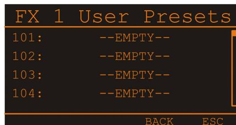
Turn the MENU/ENTER rotary encoder to select the user preset where the edited effect should be stored to. Press the MENU/ENTER rotary encoder to open the Set FX Name dialog.
