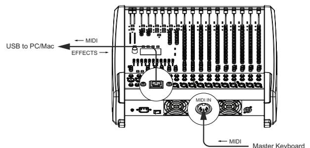
The PowerMate offers similar options for the creation of sound effects. The PC serves as an external, extremely powerful multi-effects unit. Since the signal is fed from the AUX way, the operation during mixing becomes as simple as using the internal effects of the PowerMate. The AUX way should be switched to post-mode. The effect signal generated in the PC is again added to the overall mix via USB stereo channels 1-2 and 3-4. The stereo channel faders serve as FX-return controls.
