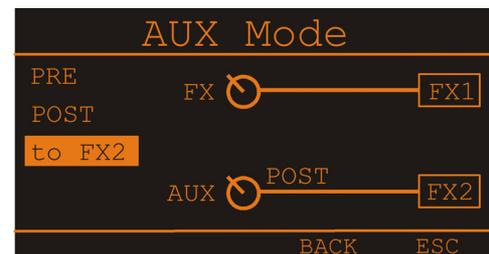
In this mode the AUX channel is used as FX 2 channel, so the AUX controls allow adjusting individual amounts of the input signals to be routed to the integrated FX 2 effects units. At the same time the FX controls allow adjusting individual amounts of the input signals to be routed to the integrated FX 1 effects units (see page 12 for details).
