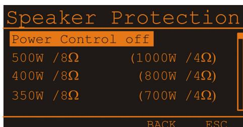
Turn the MENU/ENTER rotary encoder to select the RMS power rating of the connected loudspeaker. Each row shows the output power for 8 Ohm speakers on the left hand side, this value is also shown in the display in effect mode. Additionally each row shows the corresponding output power if an 4 Ohm loudspeaker is connected. To deactivate Speaker Protection select the entry „Power Control off“. Press the MENU/ENTER rotary encoder to
