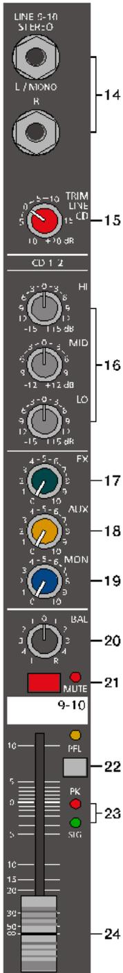
achieved at the 0 dB mark. The control offers level reduction of -10 dB and an amplification of +20 dB. This range allows the connection of most professional, semi professional, and hi-fi sound sources. For further details on how to set the TRIM LINE CD control, please refer to the description of the GAIN control in monaural channels.
