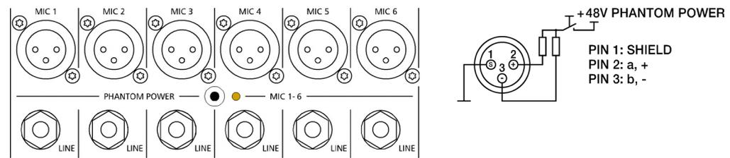
The MIC input accepts levels between -60 dBu and +11 dBu – depending on the setting of the corresponding gain control. Because of the low impedance and the switchable PHANTOM POWER the XLR input is preferred for MIC applications. Because of the higher level and impedance matching the LINE input should be preferred for connecting further mixers, effect units, keyboards etc.
