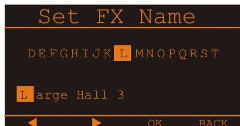
This dialog is used to change the user preset’s description. Turn the MENU/ENTER rotary encoder to the left or right to edit the highlighted character. Pressing the MENU/ENTER rotary encoder accepts the desired symbol and moves the cursor to the next character. Move the cursor to the left or to the right by pressing the ◀ or ▶ function keys. Select the ↵ symbol or press the OK function key to quit editing the name. Pressing the BACK function key returns to the menu.
