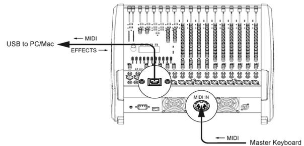
The CMS offers similar options for the creation of sound effects. The PC serves as an external, extremely powerful multi-effects unit. Since the signal is fed from the AUX way, the operation during mixing becomes as simple as using the internal effects of the CMS. The AUX way should be switched to post-mode. The effect signal generated in the PC is again added to the overall mix via USB stereo channels 1-2 or 3-4. The stereo channel faders serve as FX-return controls.
