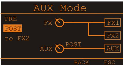
The audio signal that is present at the AUX control is tapped post volume fader and therefore affected by the fader’s setting. This mode is mainly used for establishing FX- or special monitoring mixes. Using the POST-Fader method is recommended when the mixer is also located on the stage and you have to operate it yourself. Setting
