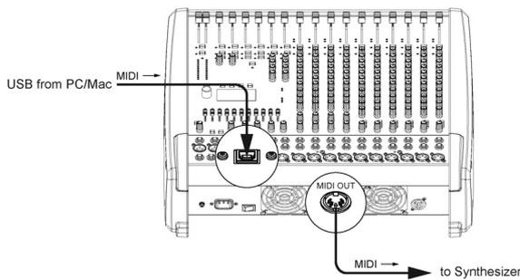
Vice versa, all MIDI data input via the MIDI IN jack are passed through to the PC, for instance to be recorded using a sequencer software application. Keep in mind that the control data for the integrated effects units, that for example can be remotely controlled via MIDI footswitch, are transmitted to the PC as well. Data error interpretation can be avoided through careful selection of suitable MIDI channels, see also "FX Control Setup" on page 23 and the documentation of your soft-
