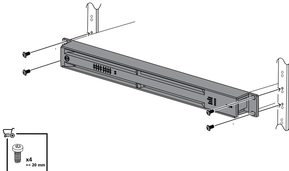
Additionally securing the amplifier by rack rails might be necessary in case you intend to transport the rack. Failure to do so may result in damage to the power amplifier as well as to the rack case.
