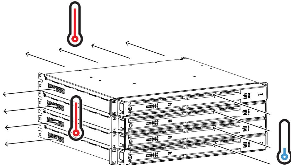
IX series amplifiers will often be installed in racks with other equipment, such as signal processors and other amplifiers. Consider that those devices accumulate heat within the rack space. An air duct of at least 30 cm between the rear panel of the IX series amplifiers and the inner wall of the cabinet or rack case is recommended. Make sure that the duct reaches up to the top ventilation louvers of the cabinets or the rack cases.
