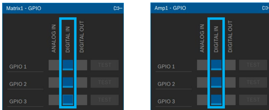
Image 34 and 35: Setting Matrix1 (left) or Amp1 (right) GPIO 1, 2 and 3 to DIGITAL IN.
