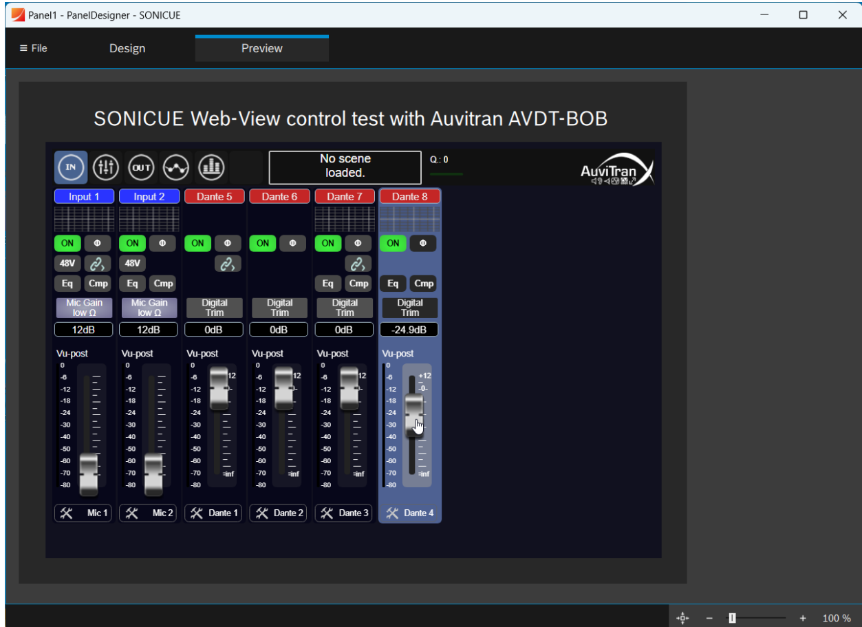
Image 11: SONICUE panel created with PanelDesigner displaying the web-UI of an AuviTran AVDT-BOB
