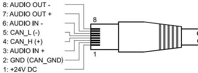
Figure 6.3: Assignment of the PCA bus connector
