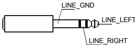
Figure 6.4: Assigning the LINE plug as audio input
