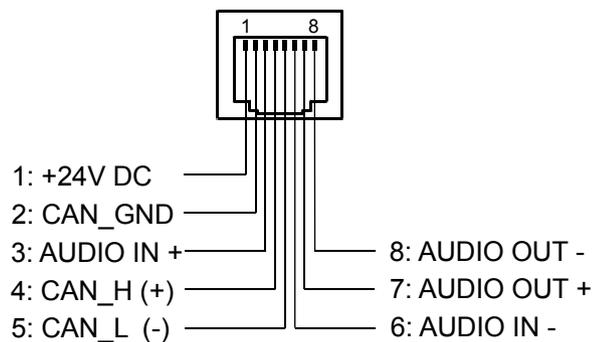
Figure 6.2: Assignment of the PCA bus interface
