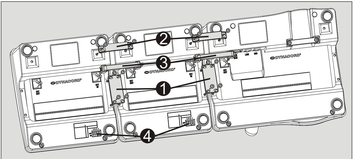
3. Mount the connecting plate (1) and connecting holder (2) with 4 and 2 screws respectively
