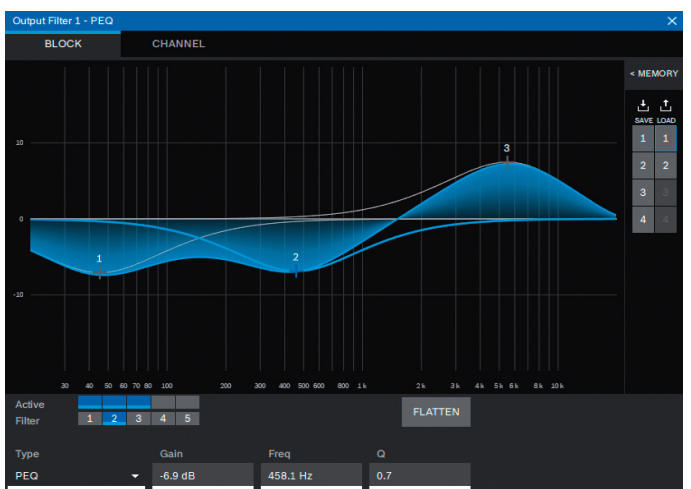
Filter adjustment in the outputs with five parametric EQs. Four settings can be stored in the Memory, between which the user can switch quickly for listening tests (Fig. 7)
