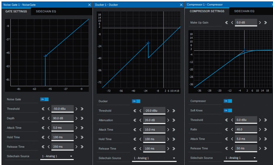
Gate, ducker and compressor with parameters and characteristic curves, in 96 kHz mode only the compressor is available (Fig. 11)
