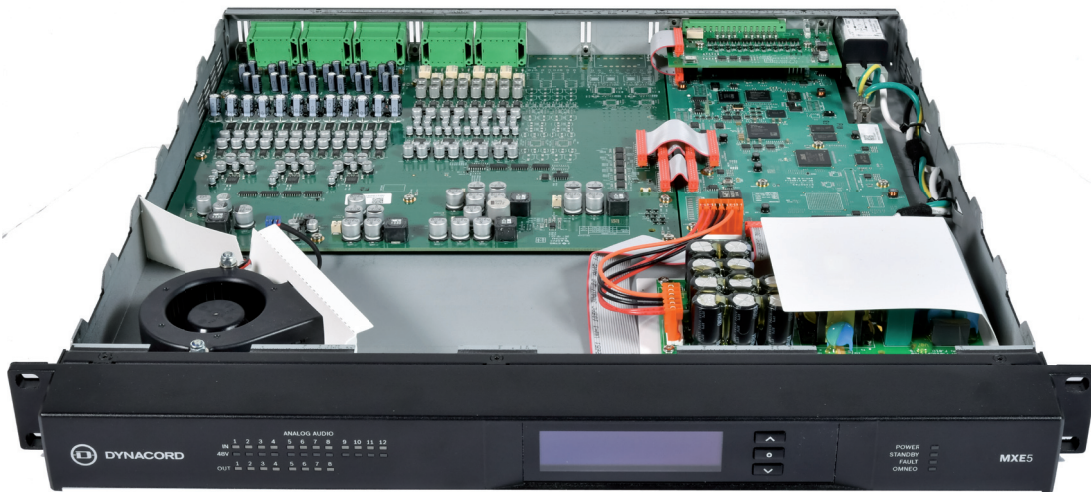
Inside view of the MXE5: rear left the large PCB with all analog inputs and outputs, right of it the DSP board and the power supply unit front right
