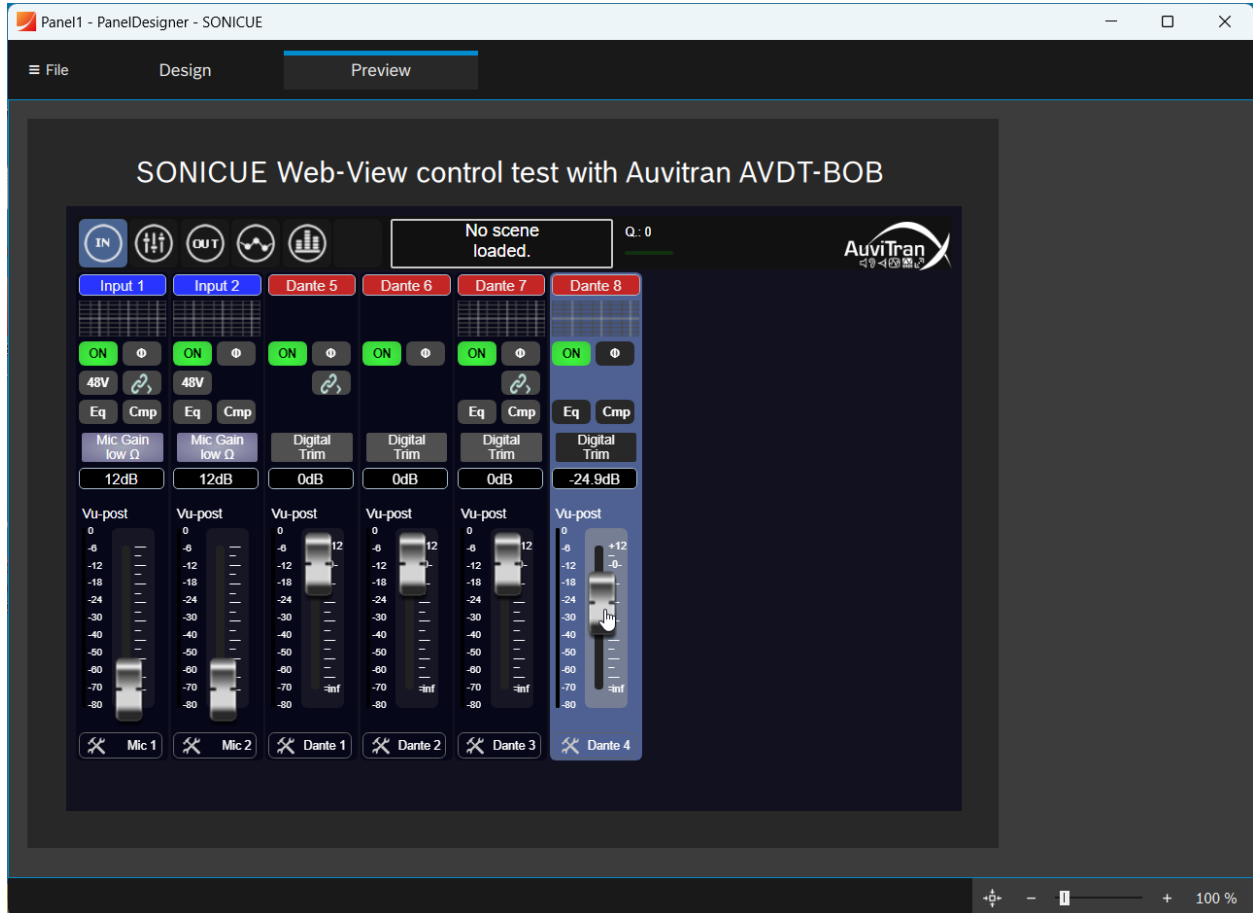
Image 11: SONICUE panel created with PanelDesigner displaying the web-UI of an Auvitrans AVDT-BOB
